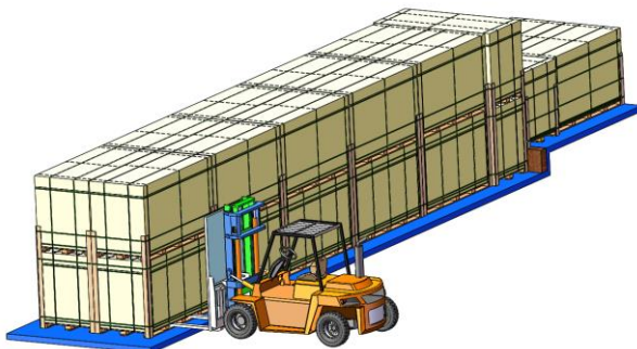
Vertical landscape package unloading with forklift
