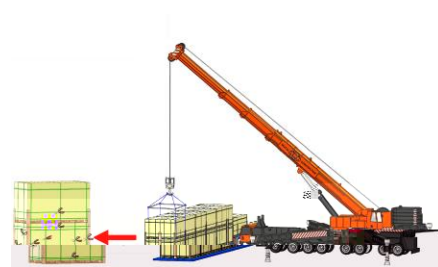
Vertical landscape package unloading with crane
