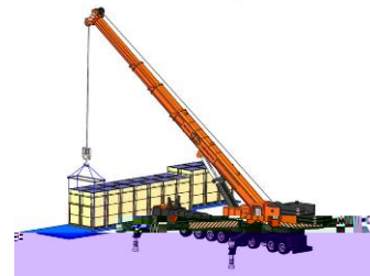
Vertical portrait package unloading with crane
